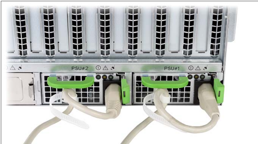
Figure 6: Cable clamps to secure the power cords
